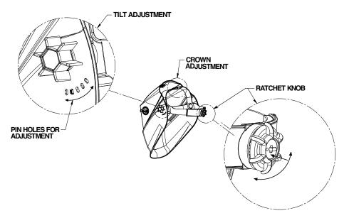
**Head Size Adjustment:** Headband tightness is adjusted by pushing in the ratchet knob and turning to adjust to desired comfort level. This knob is located at the back of the helmet. **HEAD GEAR CROWN ADJUSTMENT** is made by adjusting crown strap for vertical placement on the head and snapping the pin into the hole to lock securely in place.
