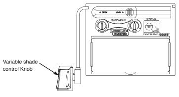
ALWAYS TEST TO BE SURE THE ADF CARTRIDGE IS CHARGED BEFORE WELDING. The TEST button is for the user to verify the ADF cartridgeis darkening properly. If cartridge is not darkening properly, replacebatteries with fresh batteries and test again before use. While welding, thearc and solar cell will keep the ADF charged.
