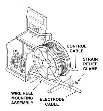
FIGURE A.3 - LN-742 WIRE FEEDER TO LINCOLN POWER SOURCE - CONNECTION DIAGRAM.
