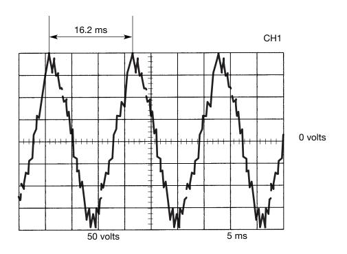
This is the typical AC output voltage generated from a properly operating machine. Note that each vertical division represents 50 volts and that each horizontal division represents 5 milliseconds in time.
