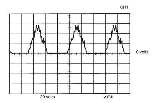
This is NOT the typical CV output voltage waveform. One output diode is not functioning. Note the "gap" in the waveform. One output diode was disconnected to simulate an open or nonfunctioning output diode. Each vertical division represents 20 volts and each horizontal division represents 5 milliseconds in time.
