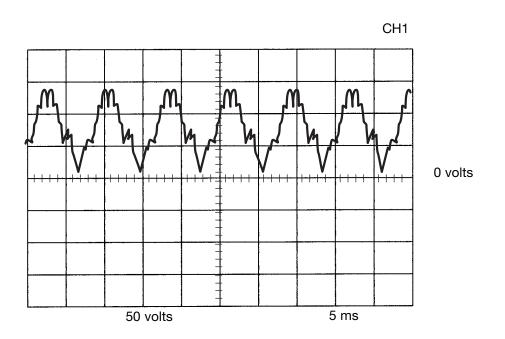
This is the typical DC output voltage generated from a properly operating machine. Note that each vertical division represents 50 volts and that each horizontal division represents 5 milliseconds in time.
