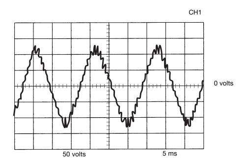
This is the typical AC output voltage generated from a properly operating machine. Note that each vertical division represents 50 volts and that each horizontal division represents 5 milliseconds in time.
