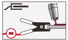
For best performance, connect the work (-) sense lead close to the welding arc.
