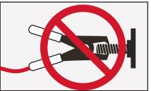
**DO NOT** connect either sense lead to a welding stud as this may result in erratic arc or increased spatter.
