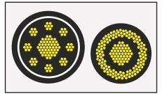
For configurations with excessive inductance, use Lincoln Electric<sup>®</sup> patented coaxial welding cables.
