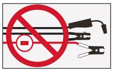
**DO NOT** route sense lead cable close to high current welding cables as this may distort the sense lead signal.
