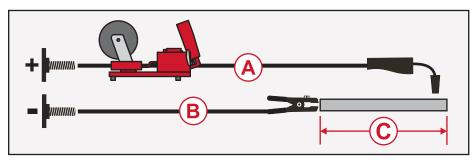
The total length of the welding current loop (A+B+C) should be minimized to reduce inductance.
