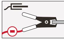
A work (-) sense lead is optional and should be connected directly to the workpiece without being in the path of current flow.
