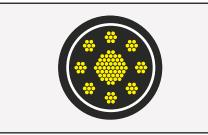
Lincoln Electric<sup>®</sup> coaxial cables combine the positive and negative welding leads into one cable to minimize cable inductance.
