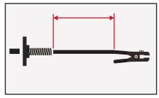
Connect the work lead to the negative stud on the power source and directly to the work piece. Maintain the shortest connection length possible.
