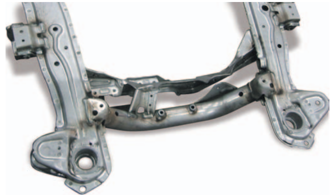
Automotive engine cradle welding – 2 mm to 2 mm (0.08 in. to 0.08 in.) lap weld and 3 mm to 4 mm (0.12 in. to 0.16 in.) lap weld at 70 ipm (1.78 mpm)
