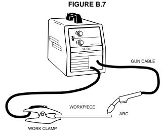
10. When no more welding is to be done, close valve on gas cylinder (if used), momentarily operate gun trigger to release gas pressure, and turn off the SP-170T.
