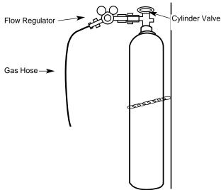
2. With the cylinder securely installed, remove the cylinder cap. Stand to one side away from the outlet and open the cylinder valve very slightly for an instant. This blows away any dust or dirt which may have accumulated in the valve outlet.
