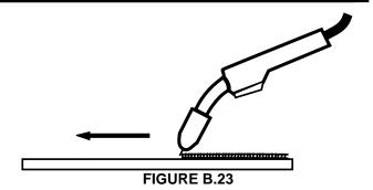
When using the GMAW process on light gauge material, weld from right to left (if you are right handed). This results in a colder weld and has less tendency for burn through.
