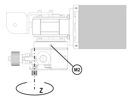
The head can be turned along Z by unfastening the three screws (M2)
