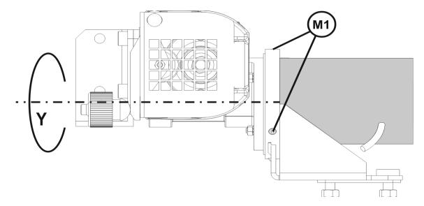
The assembly can be turned along Y by unfastening the eight screws (M1)
