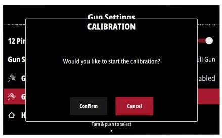
When Gun Calibration is selected, the user interface will ask the user if they would like to start the calibration. The user will select yes, and the UI will prompt to pull the trigger and wire will begin to cold feed. Once calibration is complete, the wire will stop feeding and the user interface will prompt the user that the calibration was complete and to release the trigger. NOTE: Be sure to hold the trigger during the entire calibration to avoid interrupting the calibration process.
