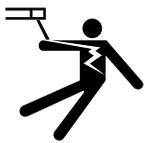
• In Stick Mode the output terminal and electrode will be electrically hot whenever the power switch is turned on.
