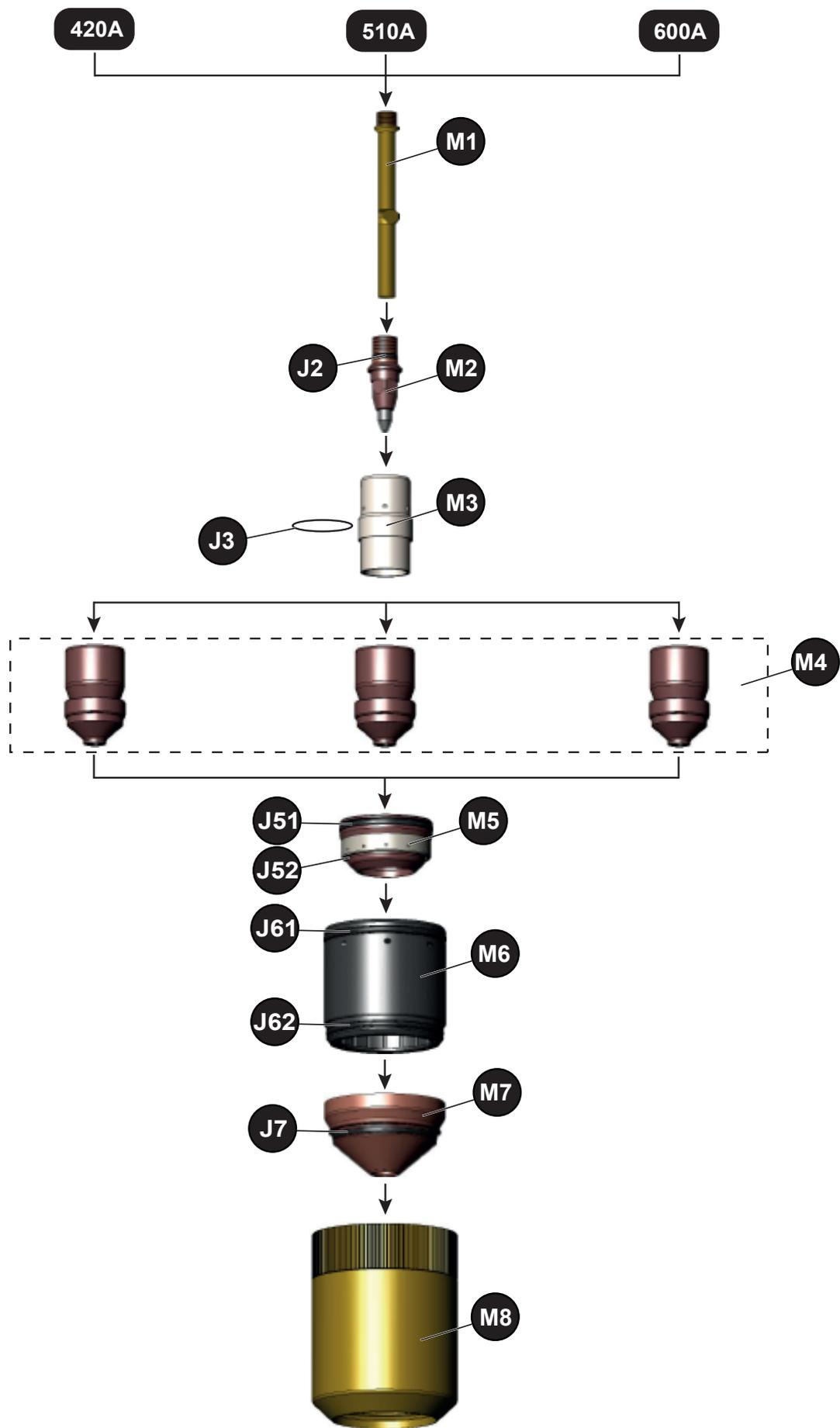
**MONTAGGIO "420A - 510A - 600A" Argon/Idrogeno**
