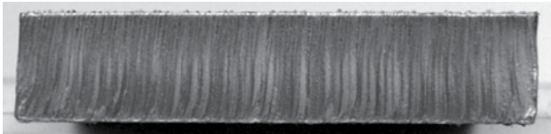
Thickness : 20mm Approximate Travel Speeds : (160 mm/min, 60A)
