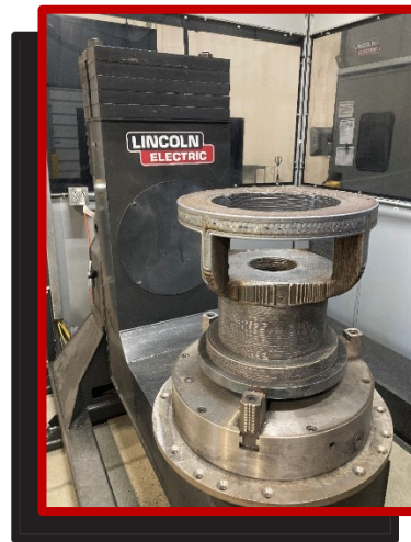
Flux Mixer Bearing Housing 22 in. Diameter by 18 in. High Low Carbon Steel - 625lbs.
