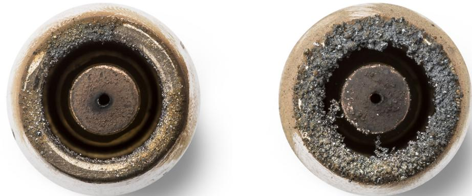
Consumables used during Standard Robotic Starting (right) versus Consumables used during AutoDrive S Touch-Retract Starting (left).
