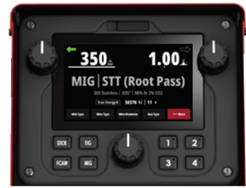
PIPEFAB™ PROCESS CONFIGURATION SCREEN WITH ARCFX® TECHNOLOGY
