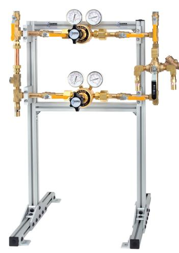
The Model 1030 is a high flow gas supply manifold intended to be attached downstream of a bulk gas system/vaporizer and which will regulate the pressure and flow of gas into facility pipelines. The manifold utilizes the Harris Model 3550-250 regulators with stainless steel diaphragms. Flow rates up to 10,000 scfh can be achieved at the nominal inlet pressure of 350 psi. The system has a 450 psi maximum rated inlet pressure.
