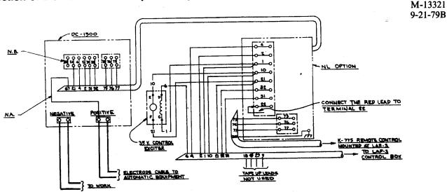
N.A. ON CODES ABOVE 5834 EXTEND LEAD AT AND CONNECT IT TO THE SLECTROSE CASLE GOING TO THE AUTOMATIC EQUIPMENT.
