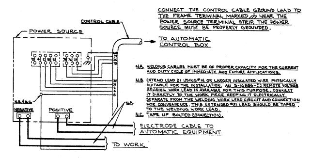
ABOYE DIAGRAM SHOWS ELECTRODE CONNECTED POSITIVE.
