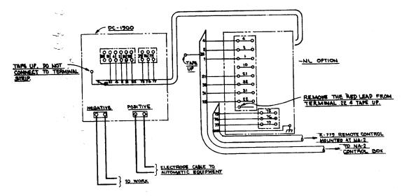
THIS DIAGRAM SHOWS THE ELECTROPS CONNECTED POSITIVE.
