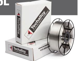
**Techalloy**® **316/316L** - For welding 316L base metals. The 2-3% molybdenum in the electrode improves pitting corrosion resistance of the weld deposit. Low carbon content reduces the possibility of carbide precipitation and intergranular corrosion.
