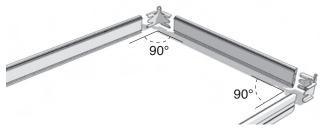
2. Slide the main frame profiles halfway over the outside corner pieces. See Figure A.3.
