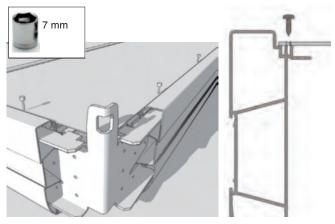
20. Slide the branding strips in the main frame profiles. See Figure A.14.
