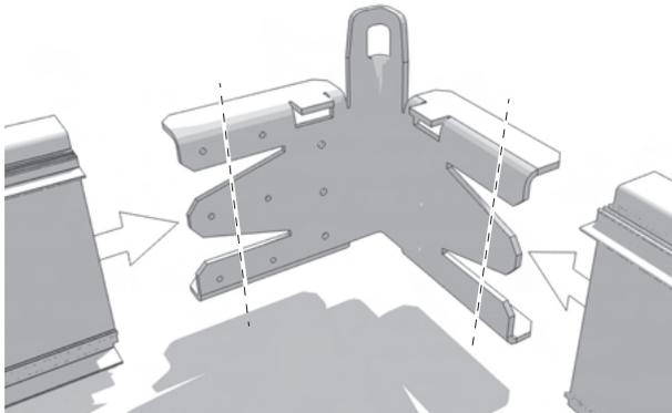
3. Place the inside corner pieces (1) and slide in the main frame profiles (2). Fasten the corner piece (3) to the main frame profiles with self-tapping screws. Use inside corner pieces as template. See Figure A.4.
