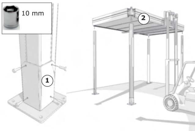
5. Make sure to position the legs as close to the corner pieces as possible, preferably using clamps. See Figure A.20.
