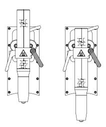
FIGURE 13 - Torch Height Adjustment
