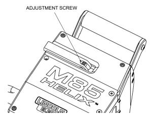
FIGURE 24 - Adjustment Screw
