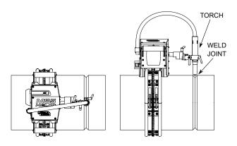
FIGURE 12 - Weld Head Placement
