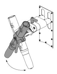
FIGURE 15 - Travel Angle Adjustment
