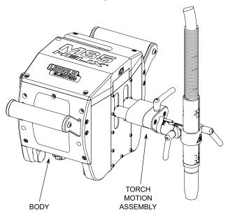
FIGURE 1 - Weld Head Compenents
