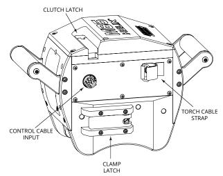
FIGURE 2 - Body Assembly (Rear)
