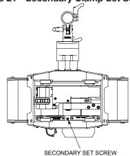
FIGURE 21 - Secondary Clamp Set Screw
