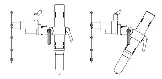
FIGURE 14 - Work Angle Adjustment
