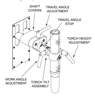
**FIGURE 3 - Torch Motion Assembly**
