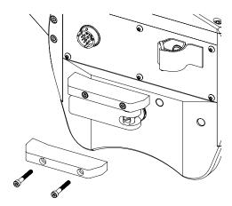
FIGURE 19 - Latch Guard Removal
