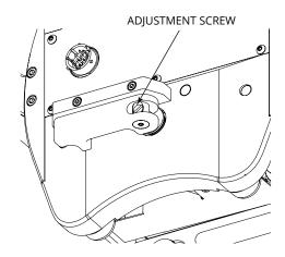
FIGURE 22 - Adjustment Screw
