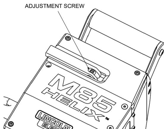
**FIGURE 24 - Adjustment Screw**
