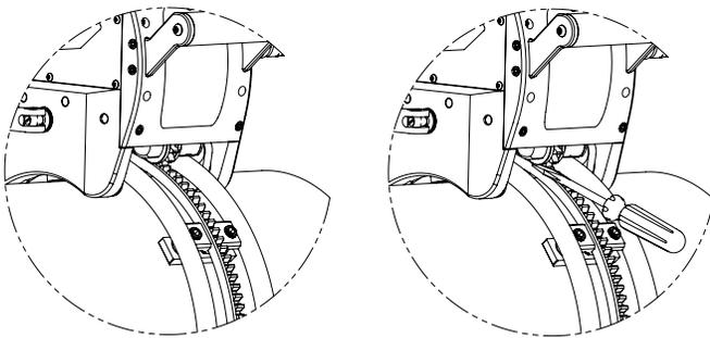
**FIGURE 23 - Track Gear Interaction**
