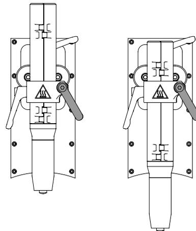
**FIGURE 13 - Torch Height Adjustment**
