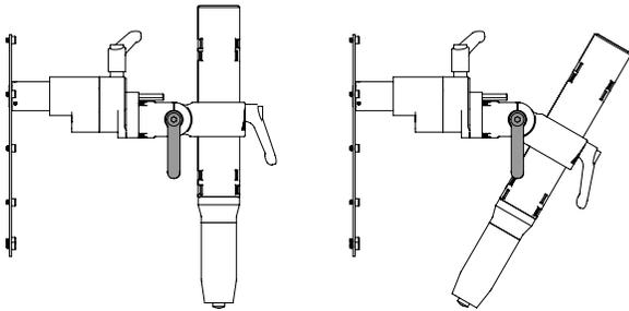
FIGURE 14 - Work Angle Adjustment
