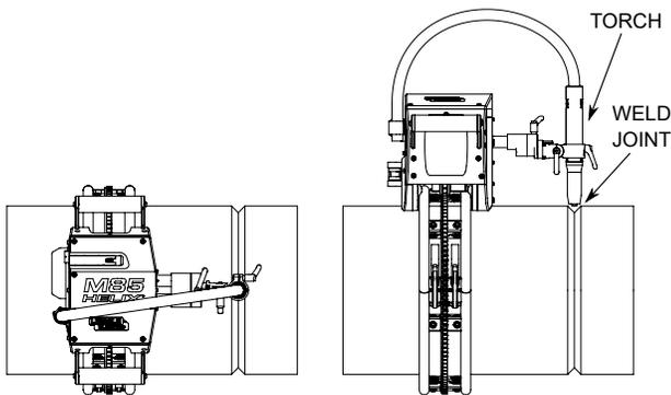
**FIGURE 12 - Weld Head Placement**
