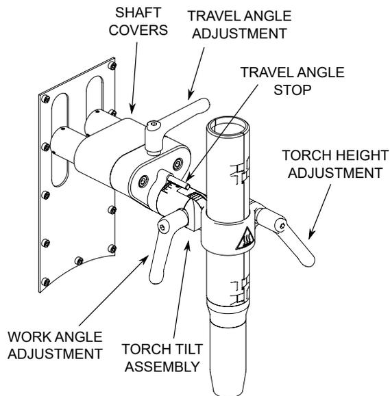
**FIGURE 3 - Torch Motion Assembly**
