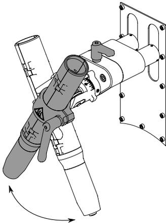
FIGURE 15 - Travel Angle Adjustment
