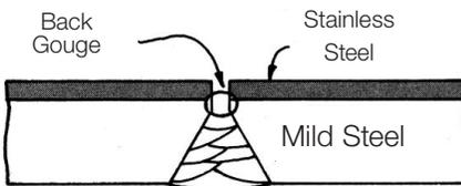
Clad steel consists of stainless steel sheet permanently bonded to mild steel plate. To join clad steel plates, first weld the mild steel with mild steel electrodes. Do not tie into the stainless cladding with the mild steel electrodes. After gouging the back-side of the first mild steel bead, weld from the stainless side using stainless steel electrodes.
