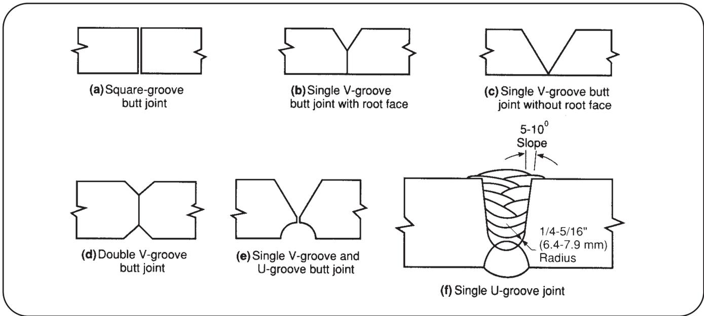
FIGURE 11 — Butt joint designs for submerged-arc welding.
