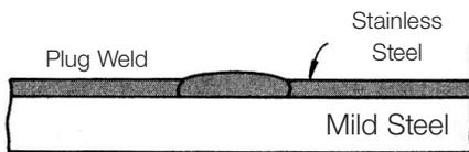
1. Large formed stainless steel sheets are plug welded at frequent intervals to join them closely to the shell.
