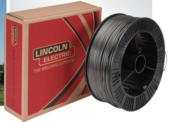
**Metalshield® MC®-110** is a low alloy metal cored wire capable of producing welds with tensile strengths of 760 MPa (110 ksi) necessary for many HSLA and quenched and tempered steels like HY-100 and ASTM 514. For an electrode designed to produce high strength, high toughness and H4 diffusible hydrogen weld deposits required in many applications, including crane fabrication – choose Metalshield® MC®-110.
