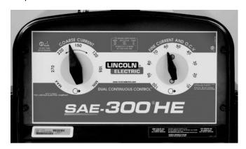
3. Use **Right Dial** (Fine Current and OCV) to Make Changes to the Arc Characteristics and Small Changes to the Output.
