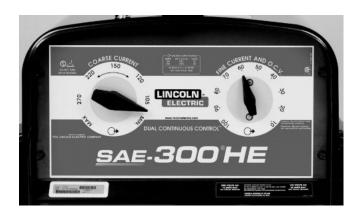
2. Set the **Left Dial** (Coarse Current) to the Desired Current. Make a small increase in current when the weather warms
