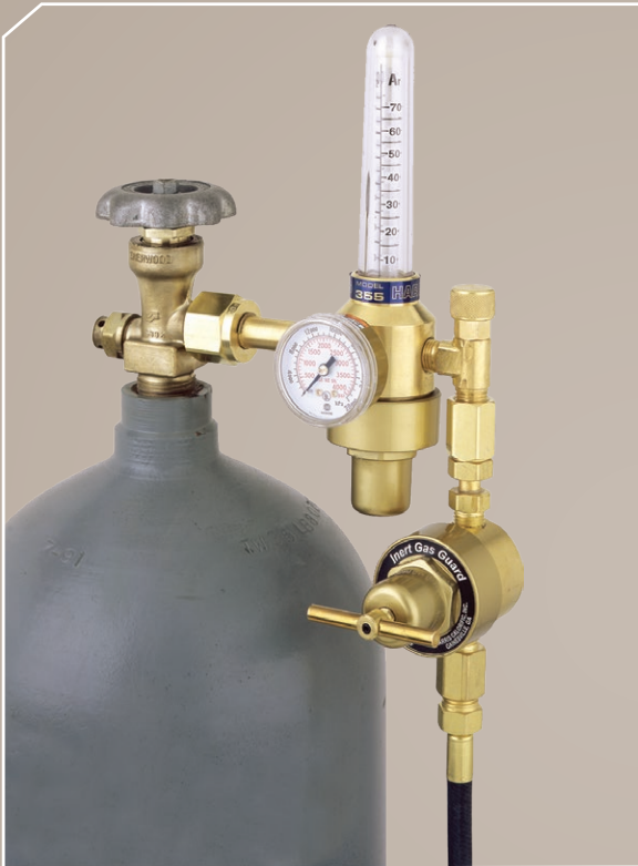
Fig. 2 A typical flowmeter regulator is a fixed pressure/variable orifice device. Pressure is set at the factory to a compensated or calibrated pressure, depending on the flow range desired and the gases being used.
