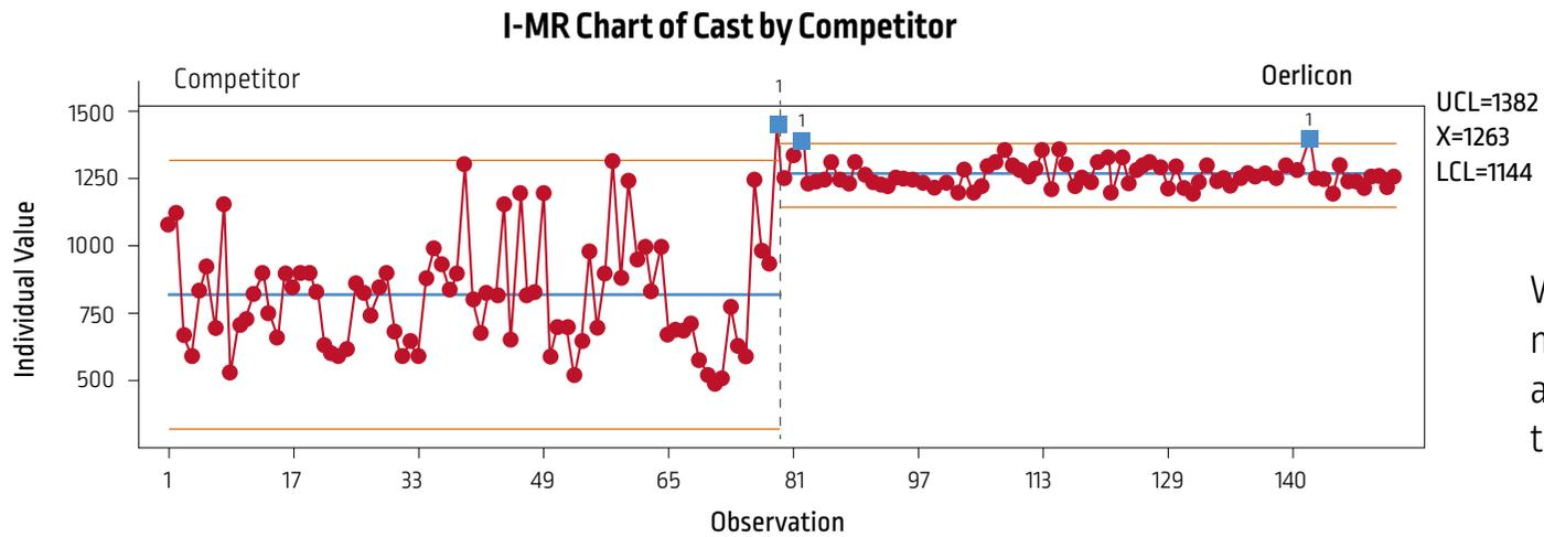
Wire features are regularly and constantly monitored: numerous checks of cast and helix values and specific attention to torsion and amplitude for drums.
