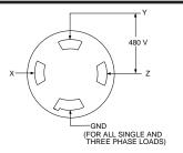
The 120V has 20 amp circuit breakers for each duplex receptacle. The 240V has 50 amp circuit breakers for each hot lead going the 240V receptacle. The 480V 3 phase circuit breakers / switch has a 3 phase, 15 amp circuit breaker.
