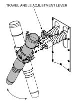
The travel angle adjustment lever serves two functions. First, it enables the operator to adjust for lead and lag - see Figure 7: Travel Angle Adjustment on page A-7. Second, it allows the torch to be moved in and out - see Figure 8: Torch In / Out on page A-7. This can vary depending on the length of the rod on the torch tilt assembly. Do not tighten the travel angle adjustment lever if there is no torch holder mounted in order to avoid damaging the clamping mechanism.
