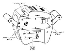
Figure 2: Body Assembly (Rear)
