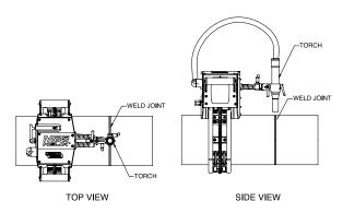
Figure 4: Weld Head Placement
