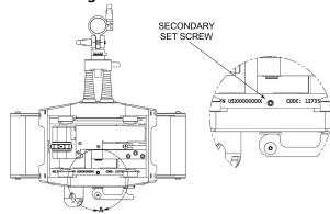
Figure 13: Secondary Clamp Set Screw
