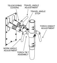
Figure 3: Torch Motion Assembly
