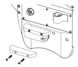
Figure 11: Latch Guard Removal
