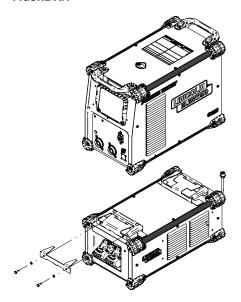
Mount the STT® Module directly to the bottom of a compatible Power Wave "S" series power source utilizing the quick lock mechanism as shown. The STT® Module will operate in harsh environments and can be used outdoors. Even so, it is important
