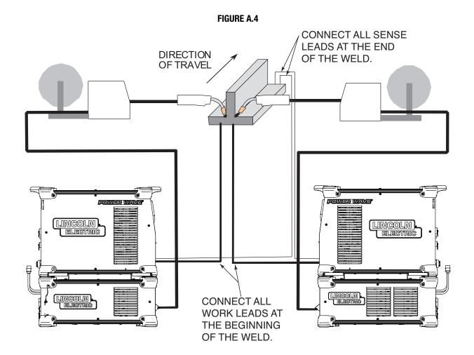
• For circumferential applications, connect all work leads on one side of the weld joint, and all of the work voltage sense leads on the opposite side, such that they are out of the current path.
