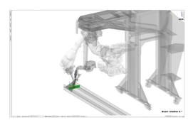
To program each tacking point automatically, click "Set all tacking points". The software will recommend a location for each tack. Tacking points can be manually adjusted, deleted, moved, or resized if necessary.
