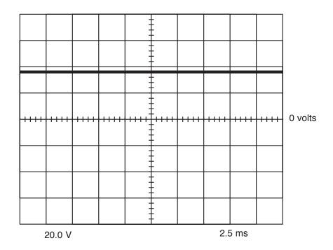
This is the typical open circuit weld output voltage generated from a properly operating machine. Note that each vertical division represents 20 volts and that each horizontal division represents 2.5 milliseconds in time.
