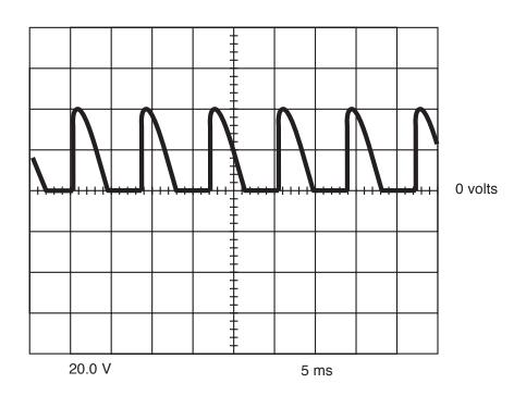
This is NOT the typical DC output voltage waveform. The output capacitors are not functioning. Note the lack of "filtering" in the output waveform. The output capacitor bank was disconnected. Each vertical division represents 20 volts and each horizontal division represents 5 milliseconds in time.
