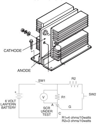
To test SCRs, construct the circuit outlined above. Resistor values are plus or minus ten percent. The voltmeter scale should be low, approximately 0-5 or 0-10 volts DC.
