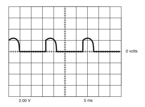
This is a typical SCR gate pulse voltage waveform. The machine was in an open circuit condition (no load) and operating properly. Note that each vertical division represents 2 volts and each horizontal division represents 5 milliseconds in time.
