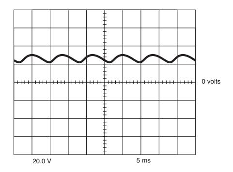
This is the typical weld output voltage generated from a properly operating machine with a load applied. Note that each vertical division represents 20 volts and that each horizontal division represents 5 milliseconds in time.
