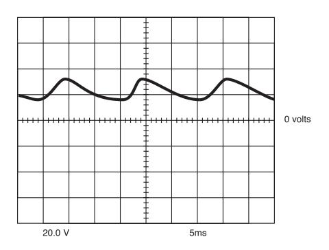
This is NOT a typical DC output voltage waveform. One output SCR is not functioning. Note the increased ripple content. One SCR gate was disconnected to simulate an open or nonfunctioning output SCR. Each vertical division represents 20 volts and each horizontal division represents 5 milliseconds in time. The machine was loaded with a resistance grid bank.
