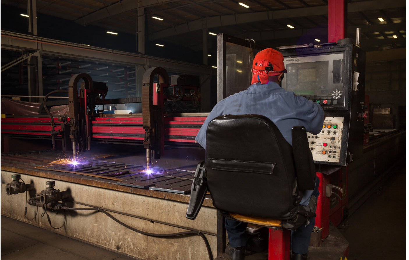
Cutting table with gantry and dual plasma torches
