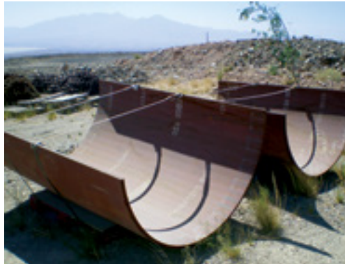
Brinell 500 Q&T liner plate installed on the compactor drums is prone to cracking and premature failure
