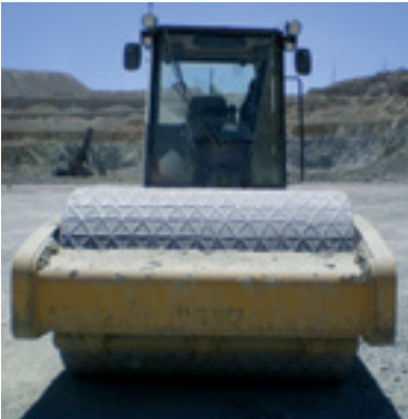
Vibratory compactors push waste rock into haulage roads to provide a level surface
