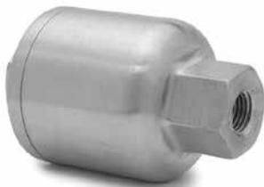
Prevents flashback in oxy-fuel gas systems. An internal check valve prevents backflow while a sintered metal filter absorbs the heat and extinguishes the flame from a flashback. Maximum flow rate - 50 SCFH
