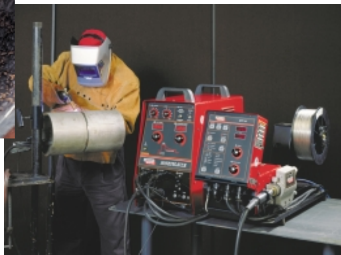
STT process using 100% CO 2 and .045 in. wire.
