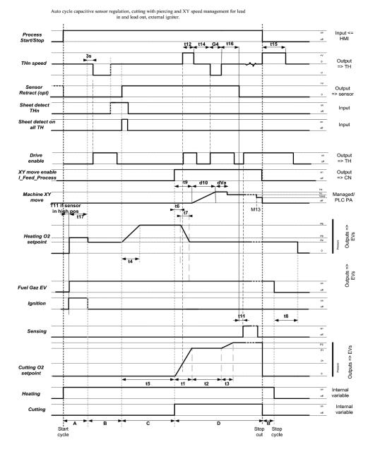
Above is a cycle for a machine with the ignition and sensing options activated
