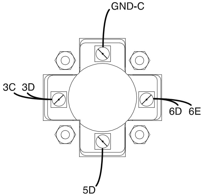
Figure F.2 – 120 / 240 VAC single phase receptacle mounting screw locations
