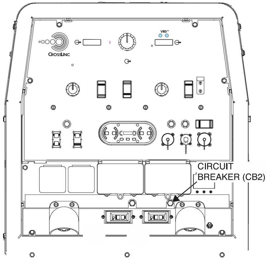
Figure F.2 – Circuit breaker (CB2) lead locations
