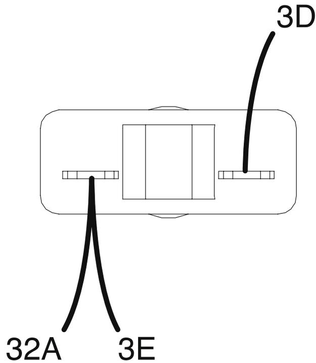
Figure F.2 – Circuit breaker (CB2) sealing boot location
