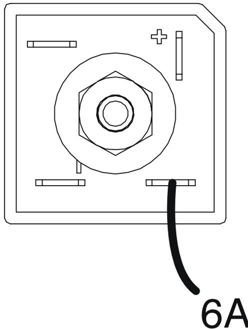
Figure F.5 – Circuit breaker (CB1) lead locations
