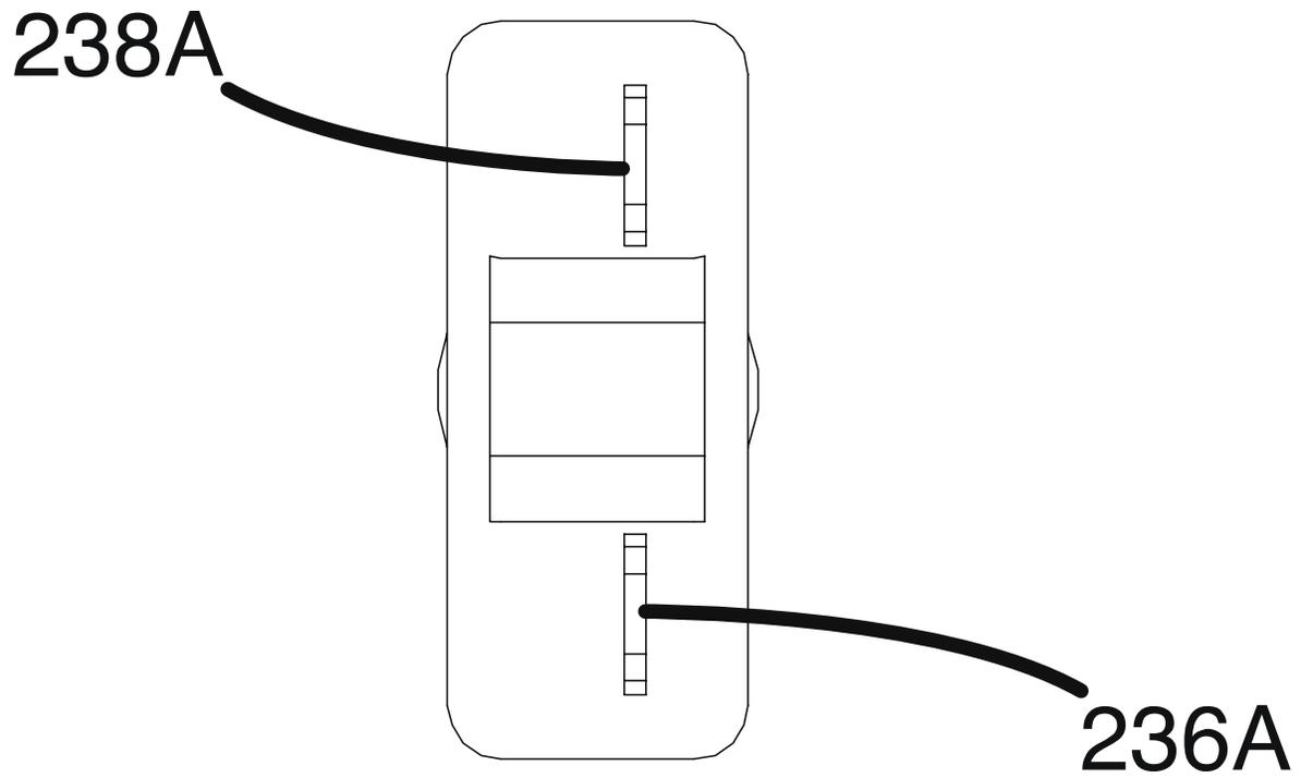
Figure F.3 – Circuit breaker (CB10) sealing boot location
