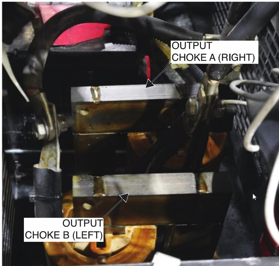
Figure F.2 – Output choke lead locations
