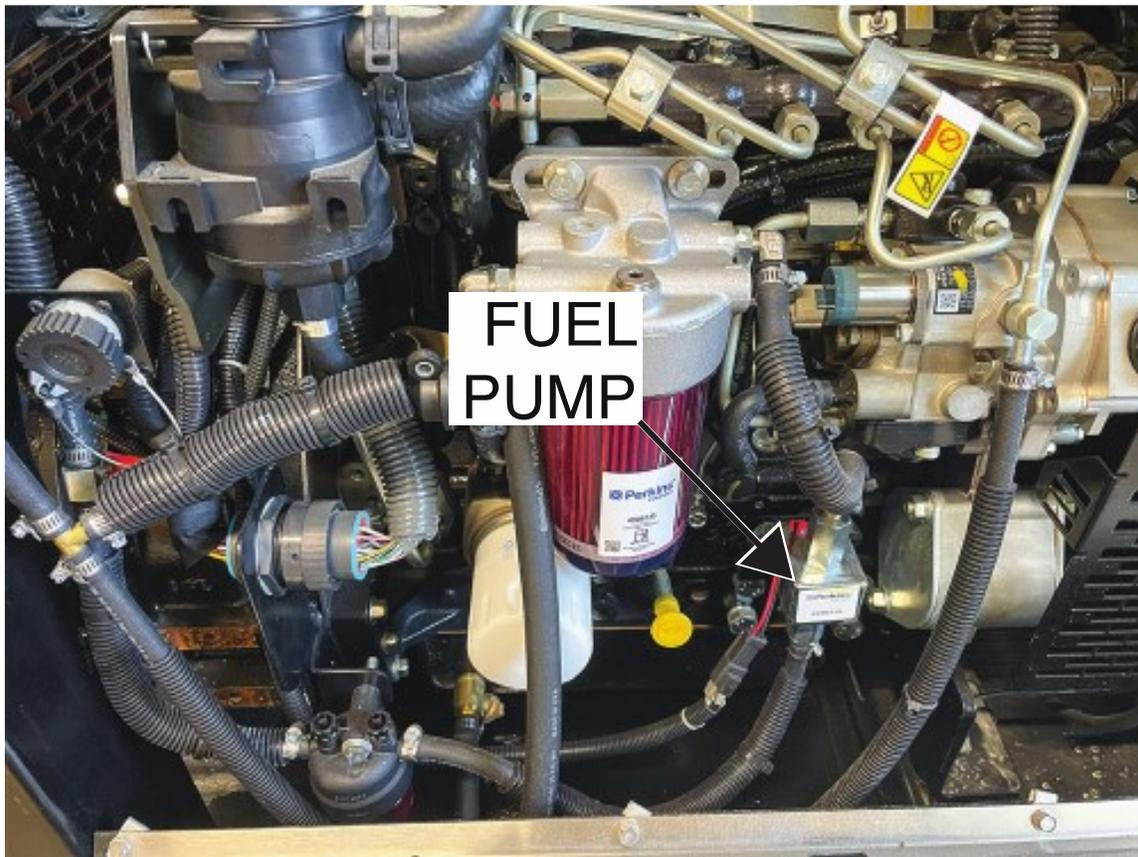
Figure F.2 – Fuel pump lead locations
