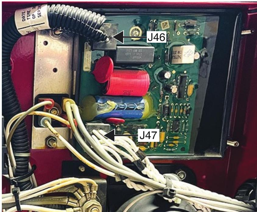
Figure F.3 – Bus board plug terminal locations
