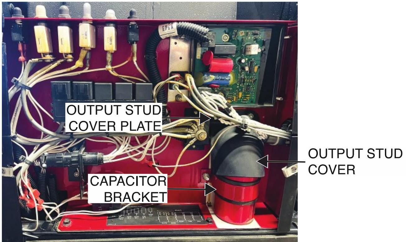
Figure F.2 – 42V capacitor lead locations
