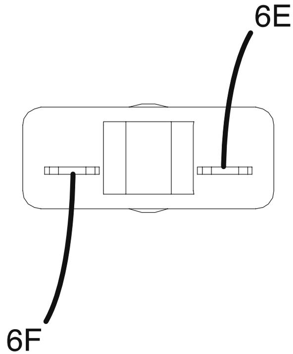
Figure F.2 – Circuit breaker (CB3) sealing boot location
