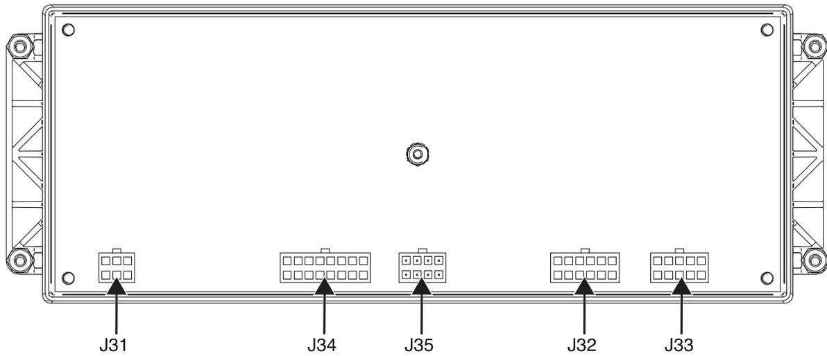
Figure F.4 – Chopper user interface board plug and terminal locations
