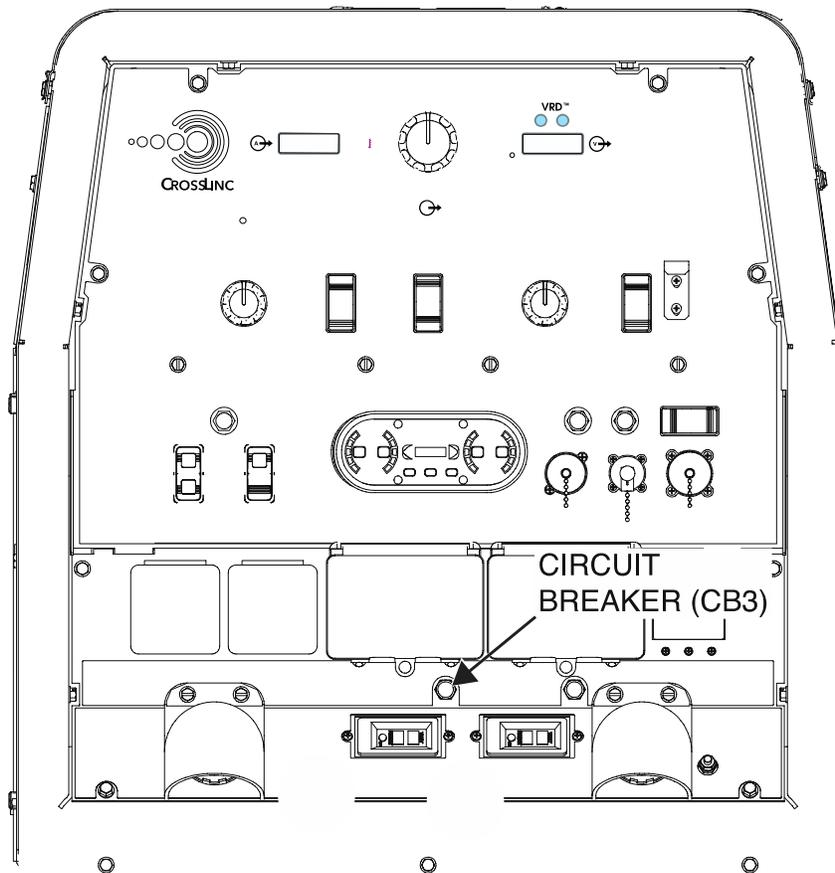
Figure F.2 – Circuit breaker (CB3) lead locations
