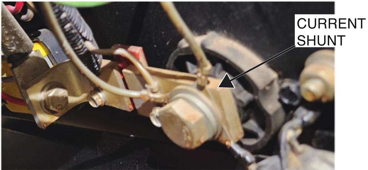
Figure F.2 – Current shunt lead locations
