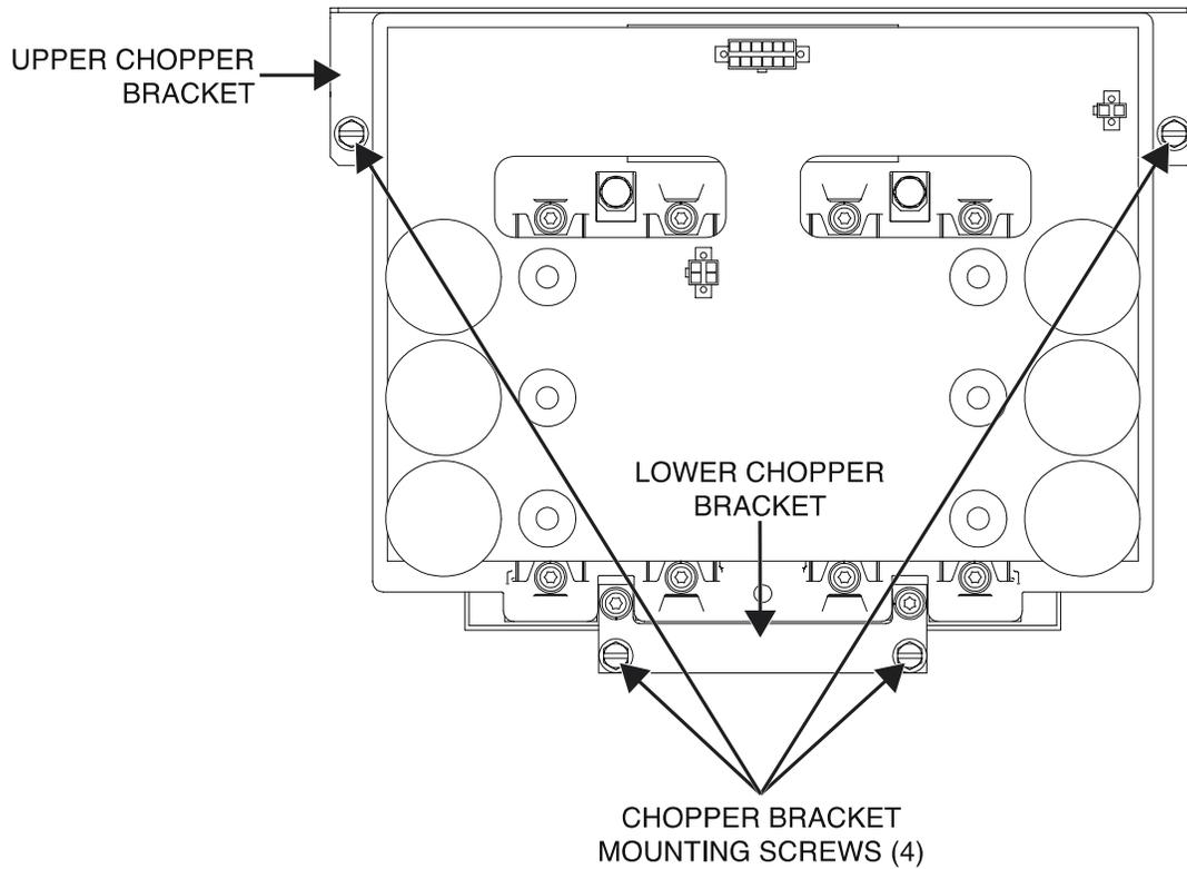
Figure F.3 – Chopper module board upper and lower bracket mounting hardware locations
