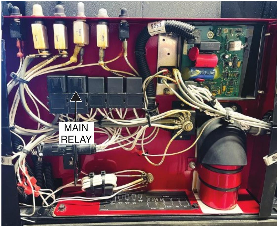
Figure F.2 – Main relay lead locations
