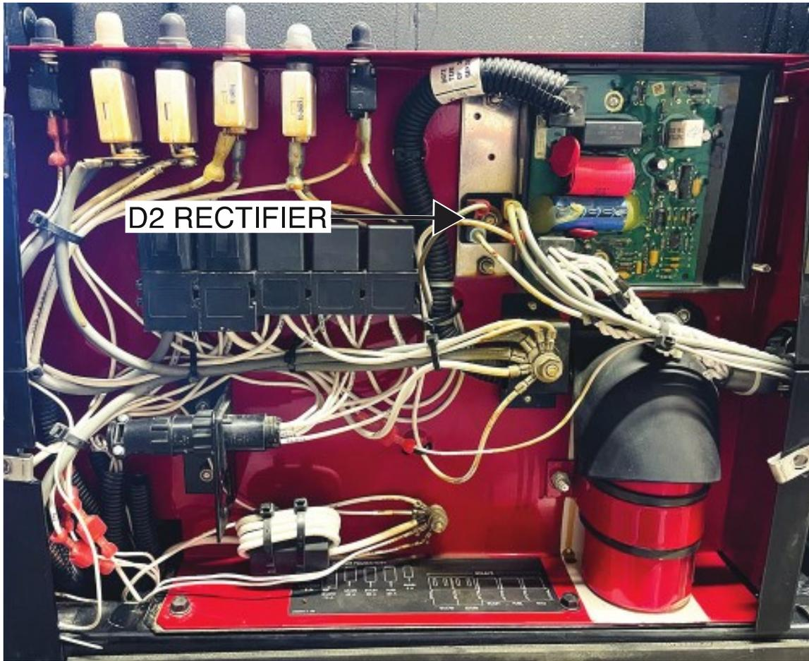
Figure F.2 – D2 rectifier lead locations
