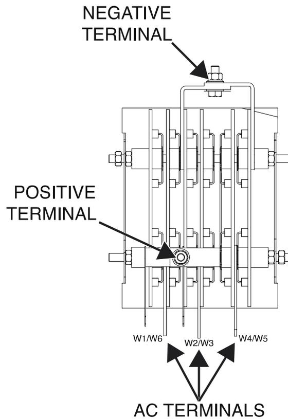
Figure F.3 – Output rectifier mounting hardware locations
