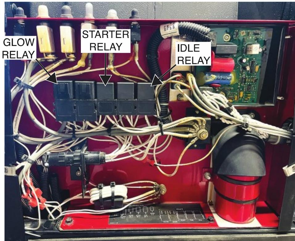
Figure F.2 – Glow relay, starter relay, and idle relay mounting nut locations
