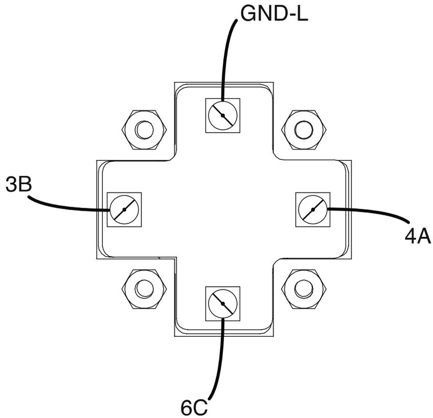
Figure F.2 – 240 VAC 3-phase receptacle mounting screw locations
