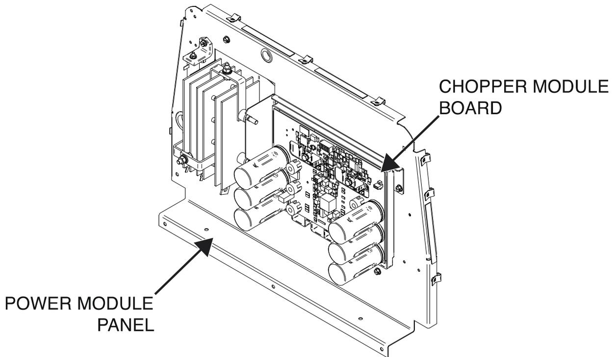
Figure F.2 – Chopper module board discharge
