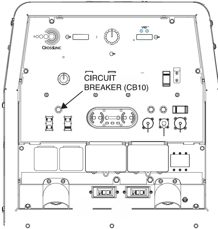
Figure F.2 – Circuit breaker (CB10) lead locations
