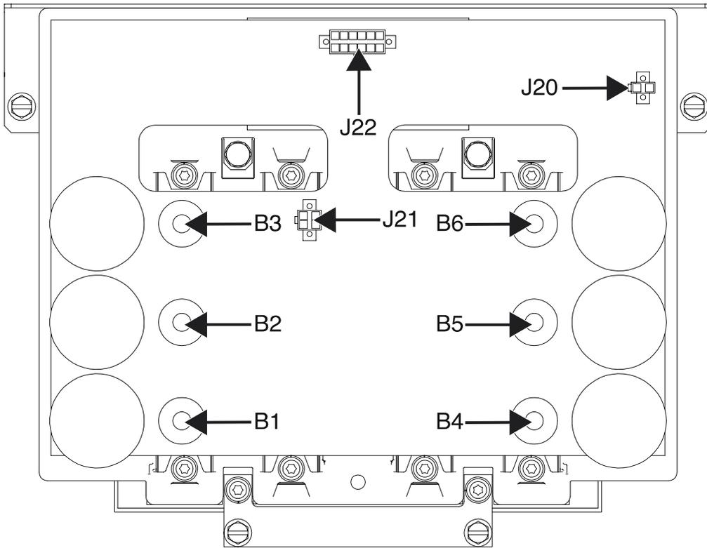
Figure F.2 – Chopper module board bracket and bracket mounting hardware locations
