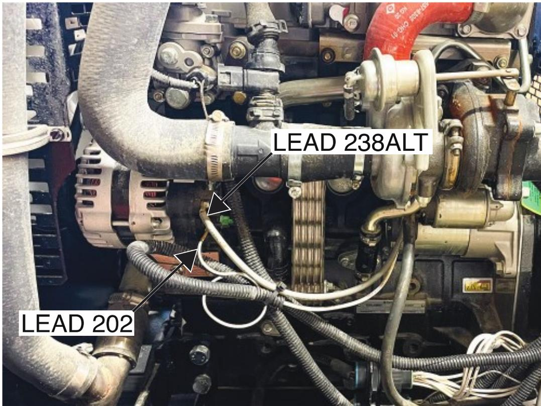
Figure F.3 – Alternator mounting hardware location
