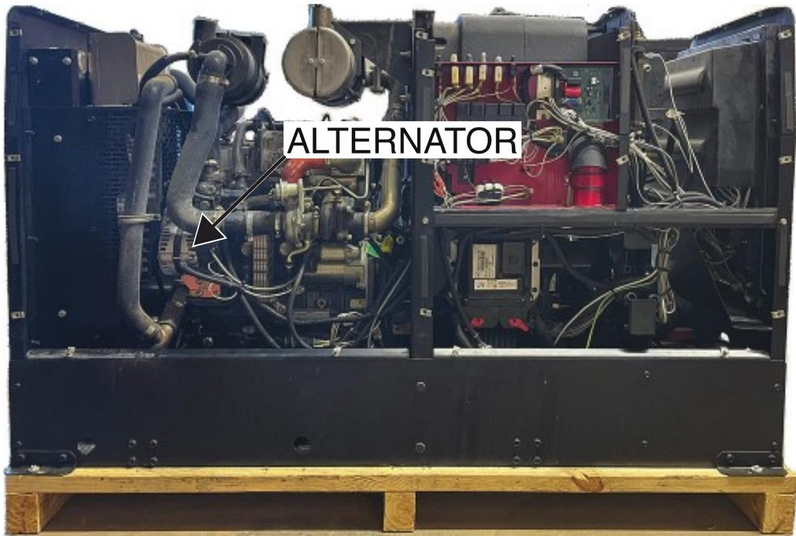
Figure F.2 – Alternator lead locations
