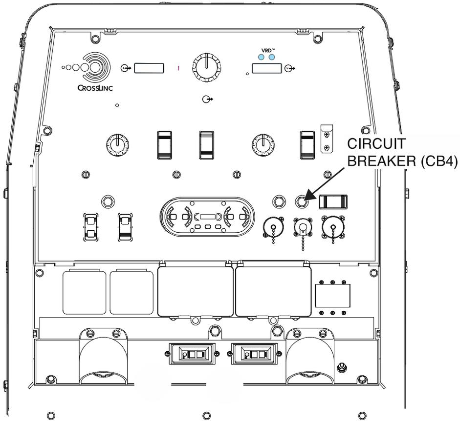
Figure F.2 – Circuit breaker (CB4) lead locations
