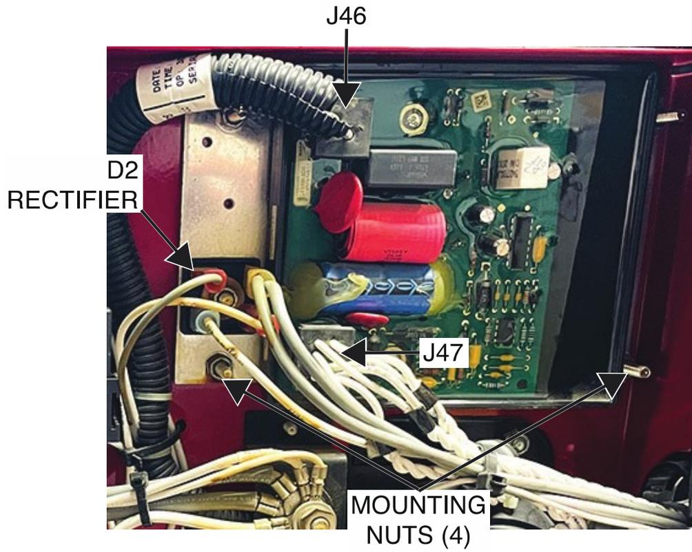
Figure F.2 – Bus board mounting hardware locations
