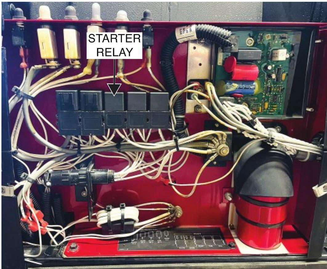
Figure F.2 – Starter relay lead locations
