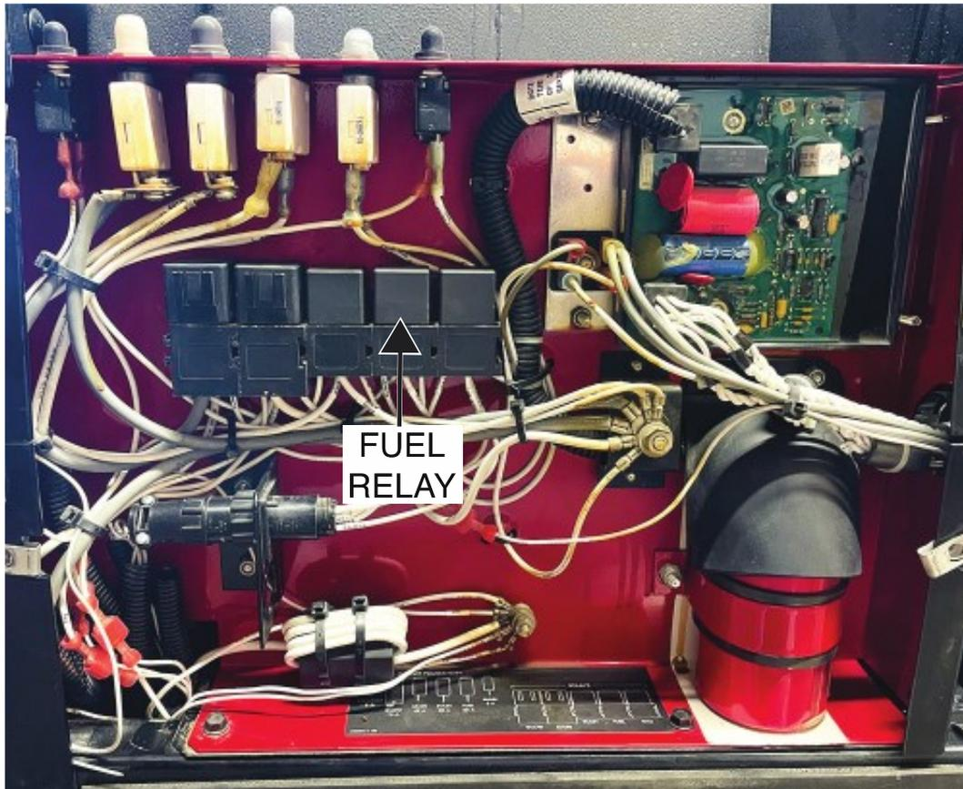
Figure F.2 – Fuel relay lead locations
