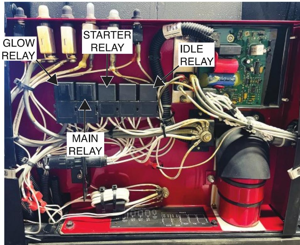
Figure F.2 – Glow relay, starter relay, idle relay and main relay mounting nut locations
