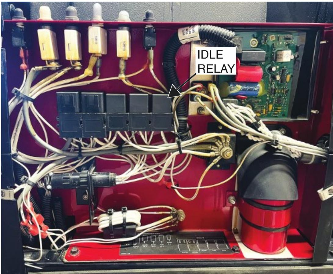
Figure F.2 – Idle relay lead locations
