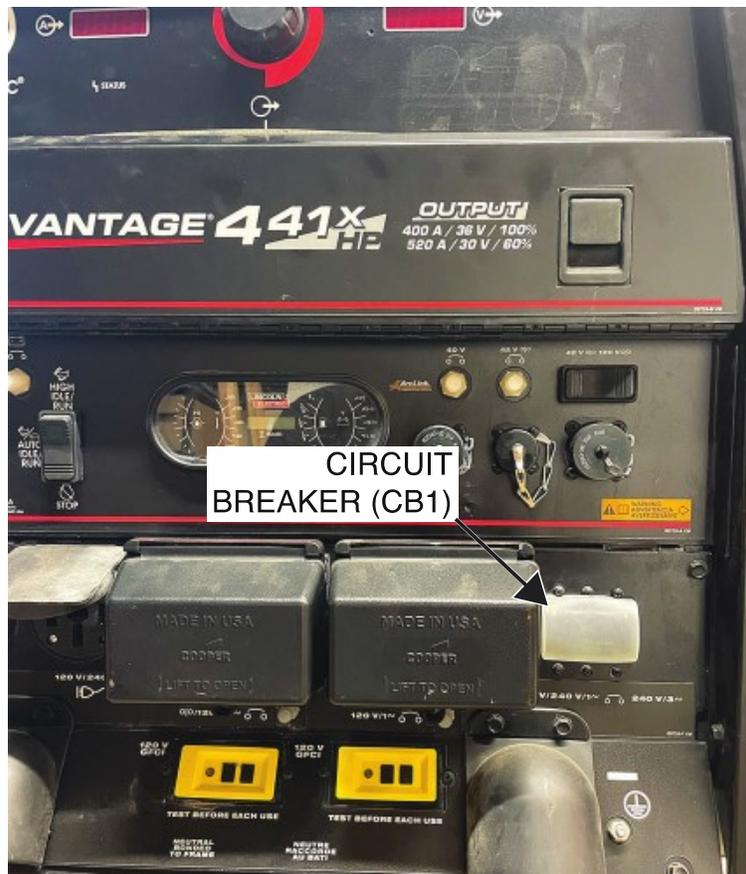
Figure F.2 – Circuit breaker (CB1) lead locations
