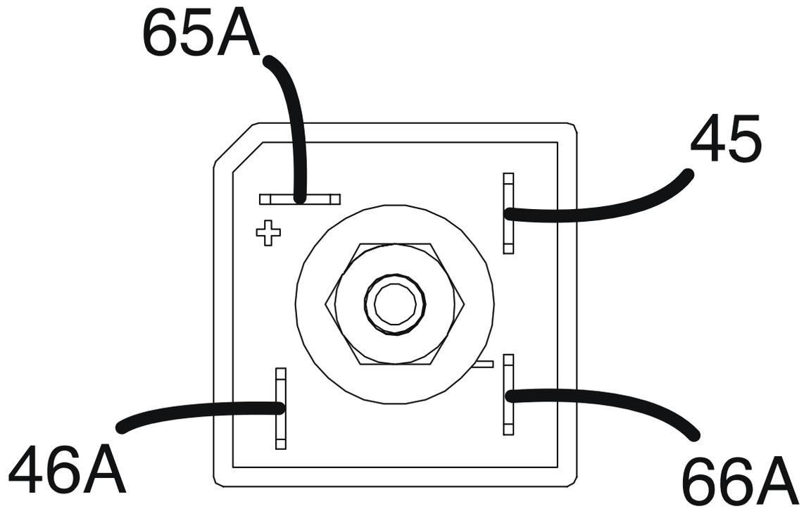
Figure F.2 – D2 rectifier mounting hardware locations
