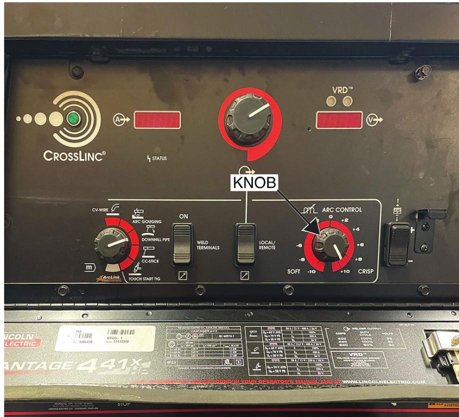
Figure F.2 – Arc control potentiometer mounting hardware locations
