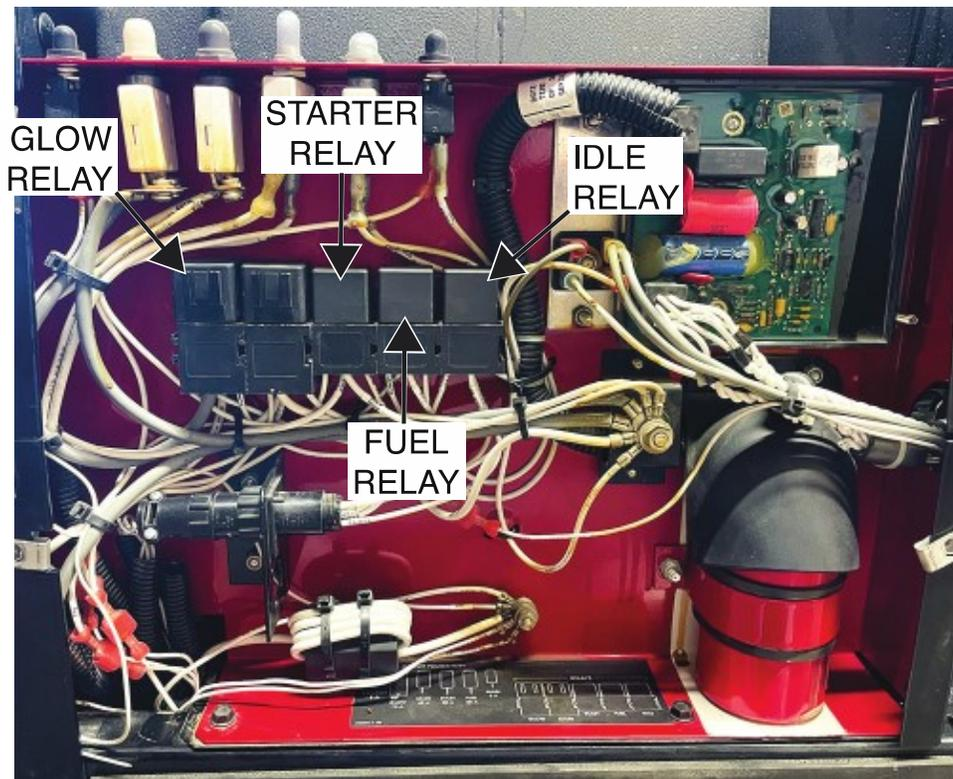
Figure F.2 – Glow relay, starter relay, idle relay, and fuel relay mounting nut locations
