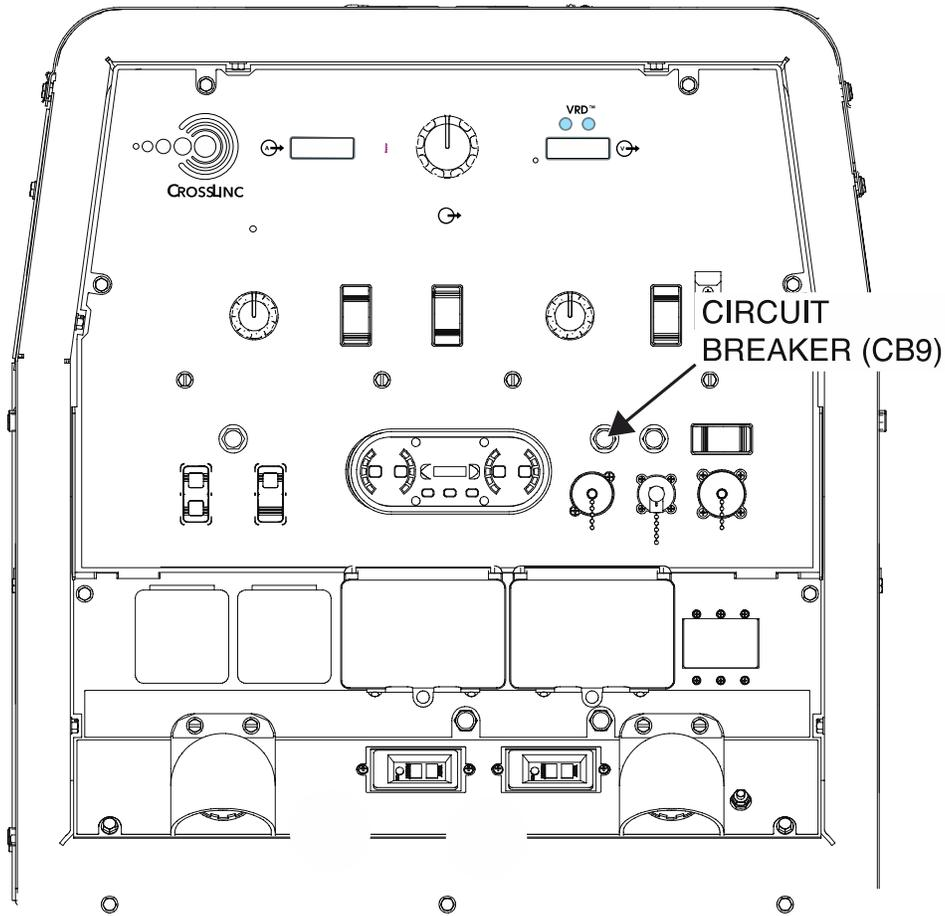
Figure F.2 – Circuit breaker (CB9) lead locations
