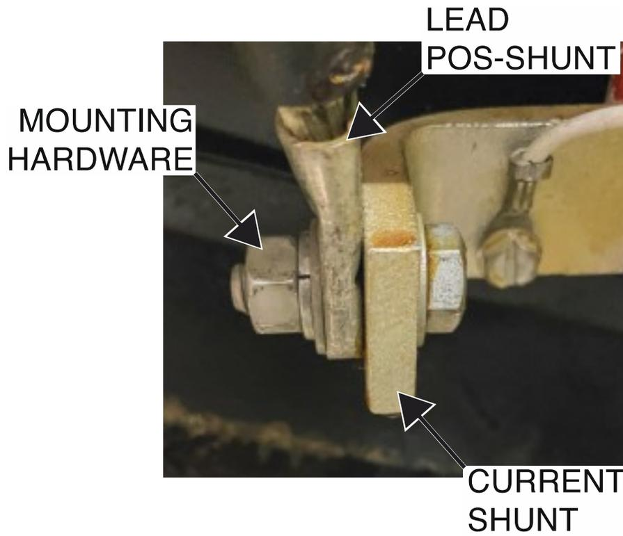
Figure F.2 – Current shunt mounting hardware location
