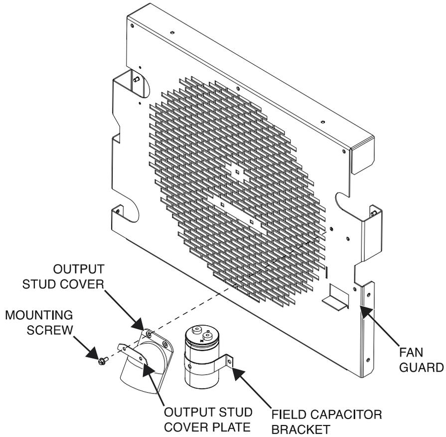
Figure F.2 – Field capacitor lead locations
