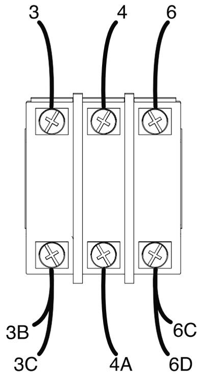
Figure F.2 – Circuit breaker (CB1) mounting hardware locations
