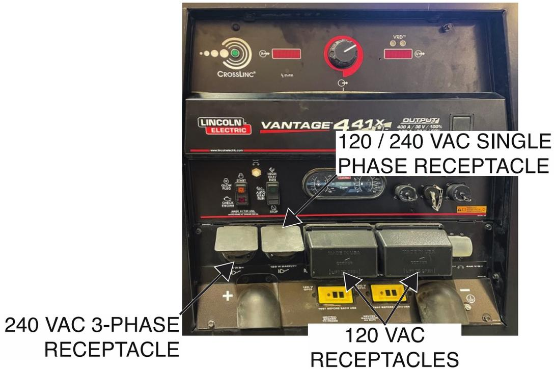
Figure F.2 – Auxiliary receptacles lead locations
