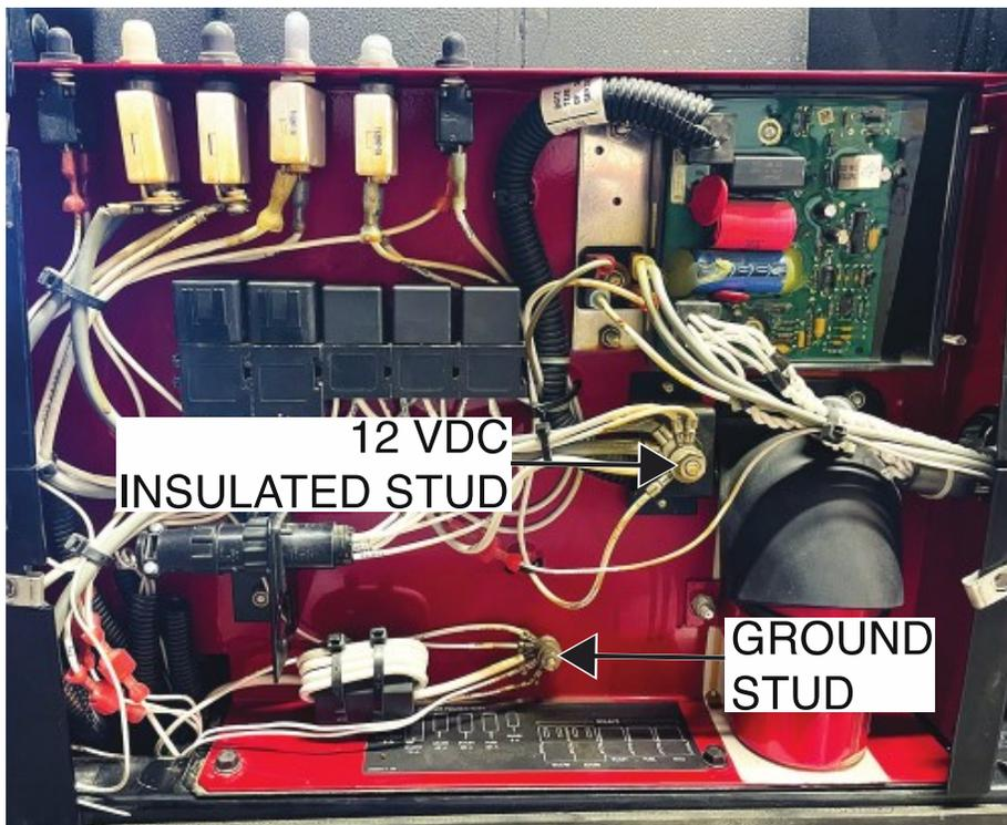
Figure F.3 – Start / glow plug switch lead locations
