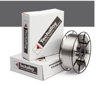
**Techalloy**® **330** electrodes are used to weld wrought and cast forms of stainless steels of similar chemical compositions, which offer good heat and scale resistance to 1800°F (980°C). However, high sulfur environments adversely affect the high temperature performance. The heat input must be kept to a minimum during welding to avoid the possibility of micro-fissuring.
