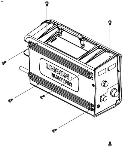
3. Remove the module from the case by lifting the front of the module approximately .25" (6 mm) and then sliding forward.
