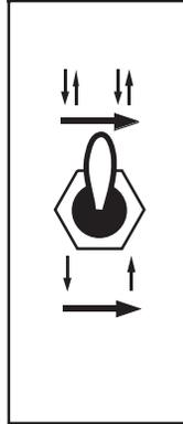
Place the toggle switch in the DOWN position for 2 Step operation or in the UP position for Trigger Interlock operation.
