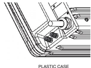
8. Slide the hose clamps on to the hoses. Trim the hoses to length so that they lay flat on the case bottom. Slide hose clamps on the hose. Slide the hoses on to the fittings on the case rear and secure with the hose clamps.
