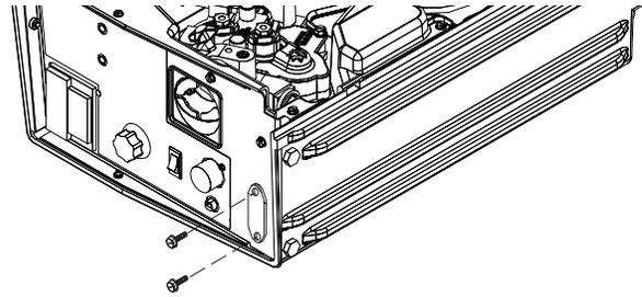
5. Install the fitting and hose assembly to the case front. Route the hoses along the bottom of the inner module and out through the cutout of the cover. Slide the module back into the case.
