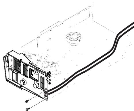
6. Secure the module to the case with the screws. (Shown in Step 2)
