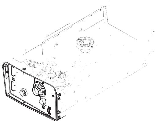
4. Use a 5/16" nut driver to remove the screws holding the water cooling cover on the case front of the inner module and on the rear of the case.
