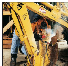
AC stick welding
