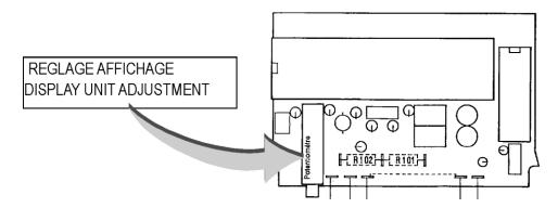
After the adjustment, press the wire feed button then the raising button, the values on the display units change.
