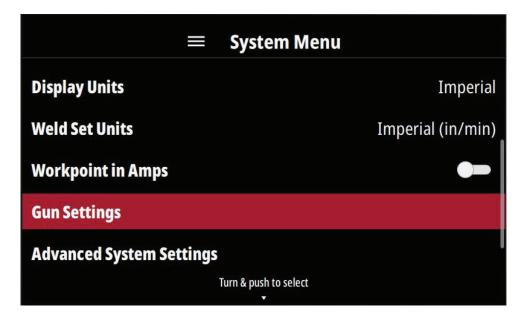
Gun settings is located in the System Menu. This is where Trigger Memory Recall, Procedure Change Method, and Aluminum specific gun settings can be found.
