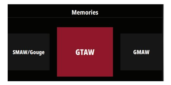
Memories can be saved for each welding process. These can be accessed by touching the applicable memory button labeled one through four.
