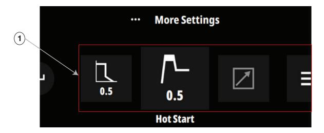
1. Advanced settings will appear here. Each weld process will have different settings. The most common advanced settings are: Pinch, Arc Force, Hot Start, Pre-Flow Time, Post-Flow Time, 2-Step/4-Step Trigger, and Ultimarc
