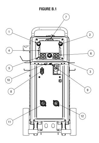
All operator controls and adjustments are located on the case front of the Power Wave (**See Figure B.1**).
