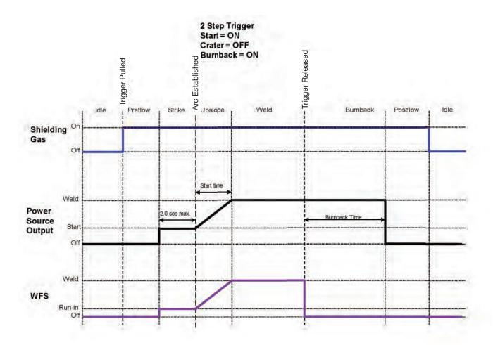
Example 3: 2-Step Trigger: Customized Arc Start, Crater and Arc End Aluminum is an example of where start, crater and burnback are commonly used to improve welding performance.
