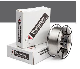
**Techalloy**® **312** is used to weld cast and wrought alloys of similar compositions. The electrode can also be used for joining hard to weld materials and dissimilar metals. Applications should be limited to 800°F (420°C). The weld deposits exhibit high tensile strength and offer some resistance to abrasion.
