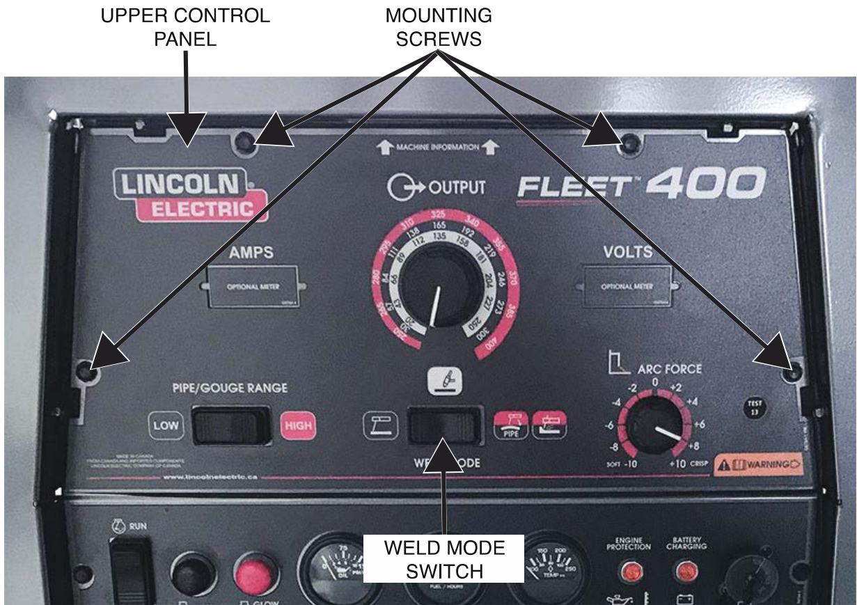
Figure F.43 – Weld mode switch leads and mounting tab locations
