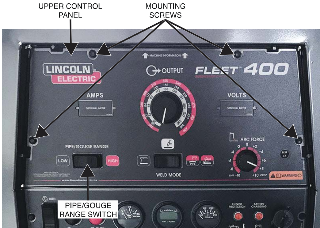
Figure F.41 – Pipe/gouge range switch lead and mounting tab locations
