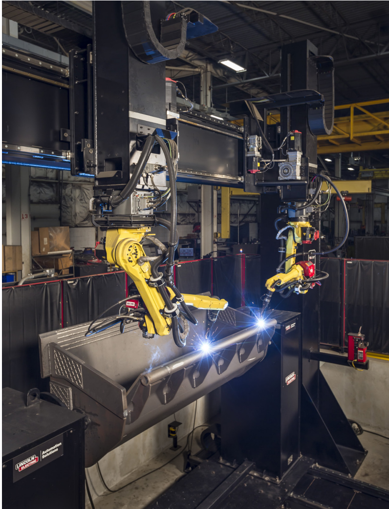
Robotic welding system with overhead crane mounted in a five-foot deep pit
