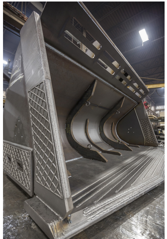
Finished bucket attachment
