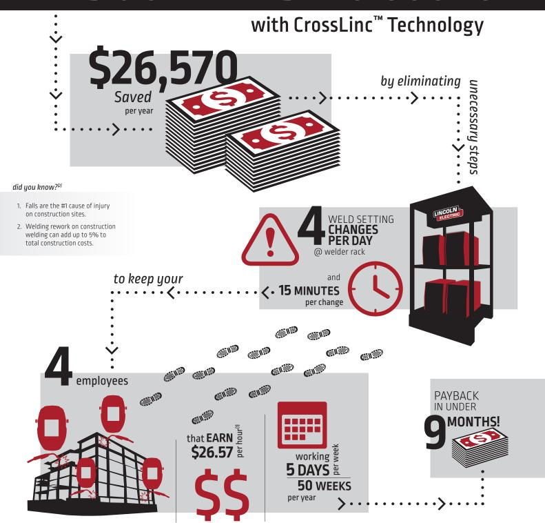
**CrossLinc™ Technology** can help you make an impact on job site safety, reduce welding costs, increase welding productivity and enhance welding quality. CrossLinc<sup>(3)</sup> enables each operator to adjust voltage at the wire feeder without a control cable, eliminating a bulky, expensive cable and multiple trips back to the welder rack hundreds of feet away.
