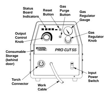
When preparing to cut or gouge, position the machine as close to the work as possible. Make sure you have all materials needed to complete the job and have taken all safety precautions. It is important to follow these operating steps each time you use the machine.
