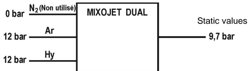
**NOTE** With **OCP 150**, if the customer uses the three methods **DUAL GAS**  $N_2 + N_2$ ,  $N_2 + Ar$  Hy and Ar Hy +  $N_2$  → two **MIXOJET DUAL** are required
