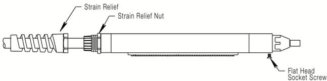
3. Remove the flat head socket screw using the 5/64" allen wrench. Grasp shield cup with one hand and barrel with other. Pull shield cup gently straight forward, until air line and solenoid connections are exposed.
