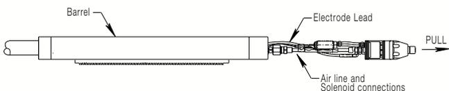
4. Using the 7/16" wrench, loosen the nut at the back of the torch head to remove the electrode lead and then unplug the electrical connector.
