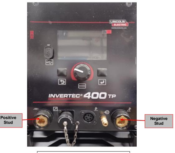
Figure 1 – Output studs location
